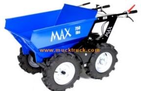
The Muck truck pedestrian dumper is designed and built in the United Kingdom and delivers obvious productivity benefits to the building/hire and landscaping industry. It can carry three times that of a conventional wheelbarrow and will transport loads of up to one quarter of a ton. A reliable Commercial grade 5.5hp Honda GX engine powers the four-wheel drive ensuring maximum traction when moving loads on wet and uneven ground.
